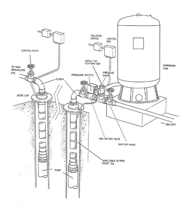
Pump connected for manual operation
